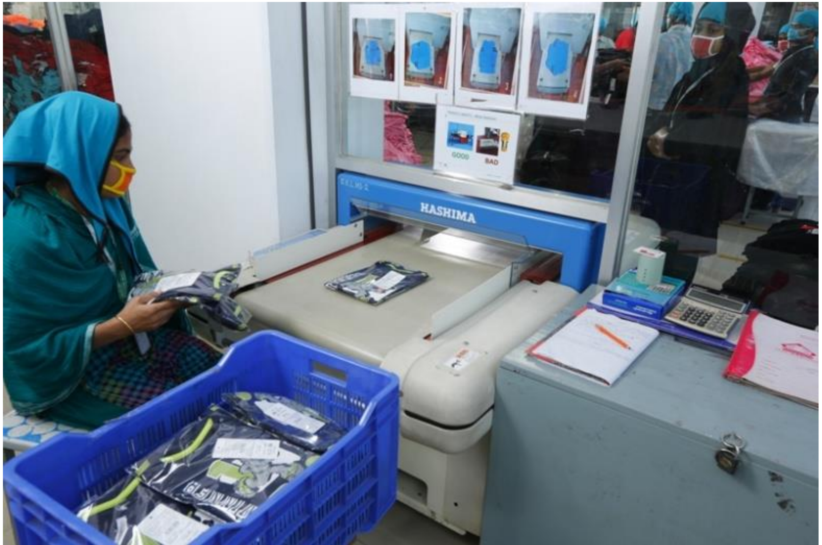
Garments passing through metal detection machine to the metal free zone Knit Garments Production Unit
